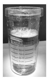
Fill the canister with water to the 0 cm line and set it into the metal bracket.
